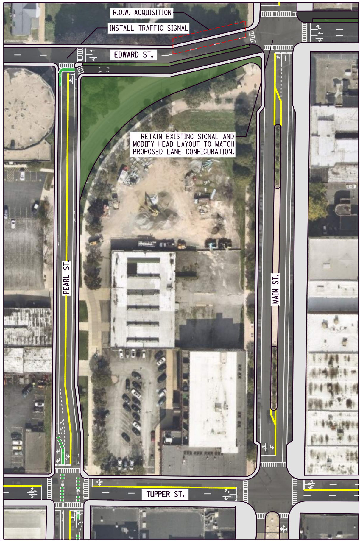
OPTION 7 PEARL ST. RE-ALIGNED PERPENDICULAR TO EDWARD ST. CONVERT PEARL ST. TO TWO-WAY TRAVEL FROM EDWARD ST. TO TUPPER ST. EDWARD ST. REMAINS ONE-WAY WESTBOUND. ROW ACQUISITION REQUIRED. GOODELL ST, ALTERNATIVE 3 SHOWN.
