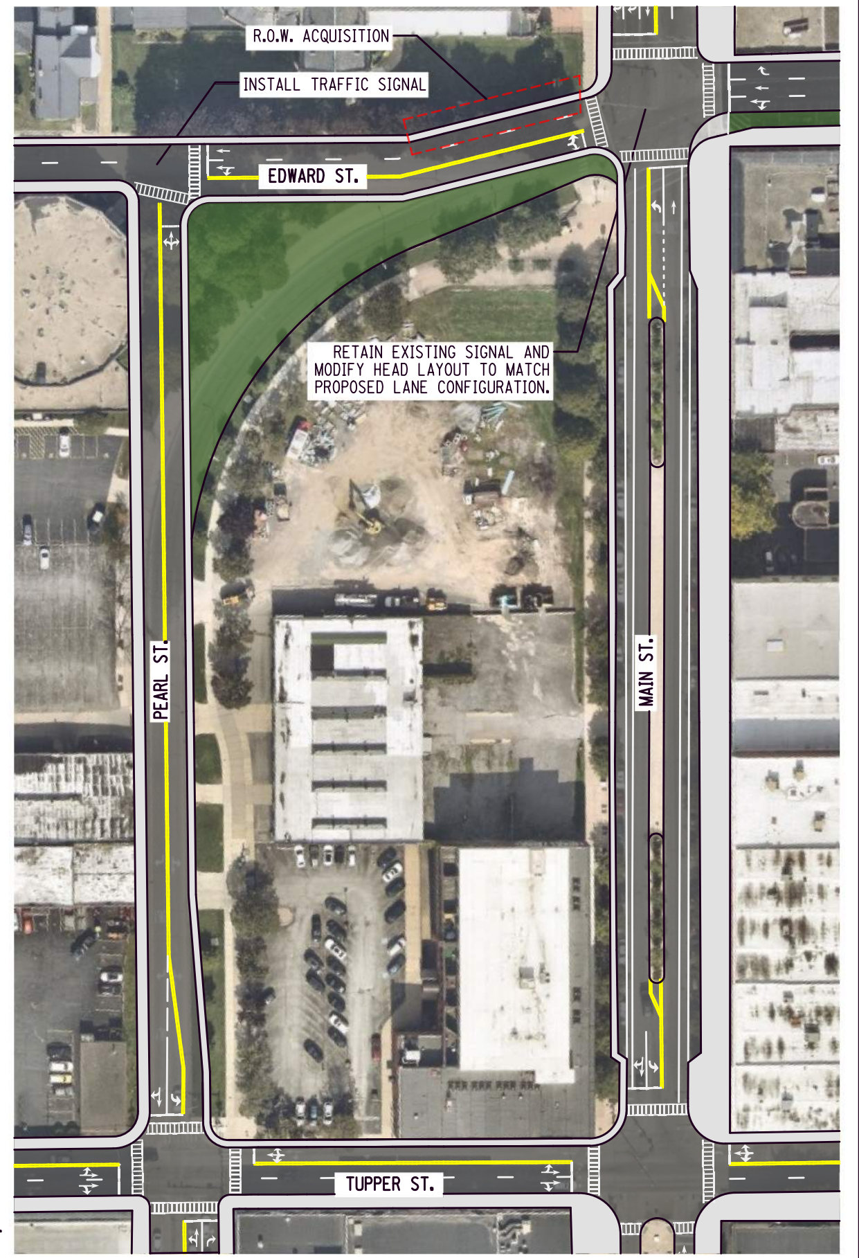
OPTION 8 PEARL ST. RE-ALIGNED PERPENDICULAR TO EDWARD ST. CONVERT EDWARD ST. AND PEARL ST. TO TWO-WAY TRAVEL FROM MAIN ST. TO TUPPER ST. EASTBOUND LANE ADDED ON THE SOUTH SIDE OF EDWARD ST. ROW ACQUISITION REQUIRED. GOODELL ST, ALTERNATIVE 3 SHOWN.
